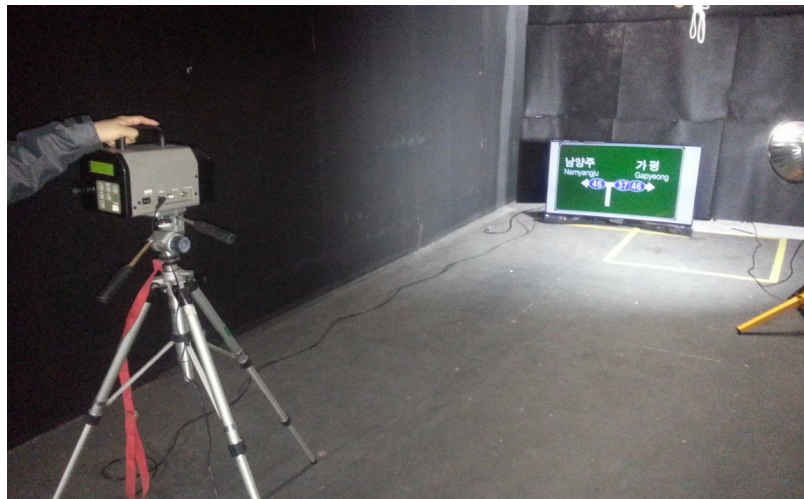
Figure 13. Luminance Measurement using the Dot Luminance Meter
