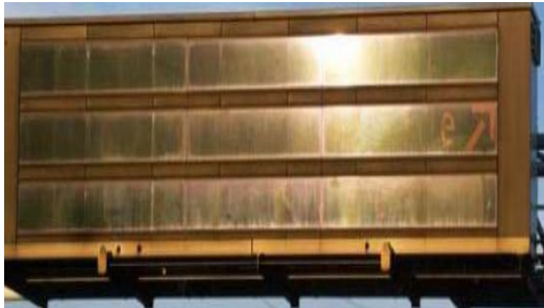
Figure 16. VMS Visibility Degradation due to Sunlight [10]
